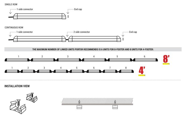
1. Position the metal clips for installation.
