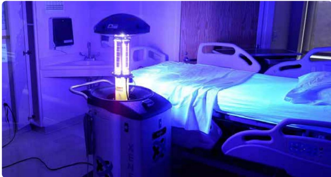
Hospital robots are disinfecting with UV-C
